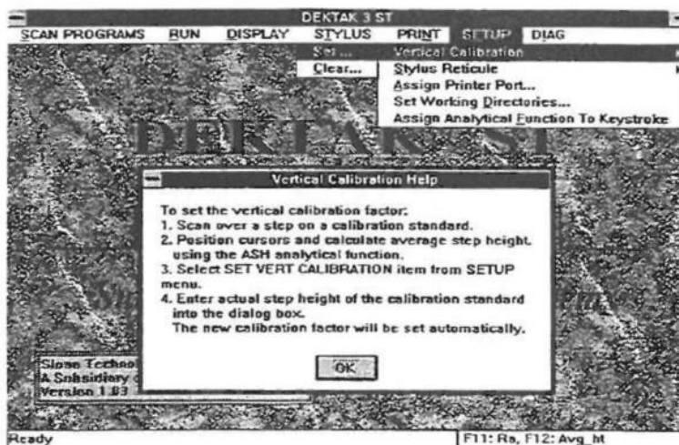
Figure 10 - 1 Vertical Calibration Set-Up
