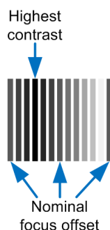
Figure 3-62 Best focus determination by microscope
